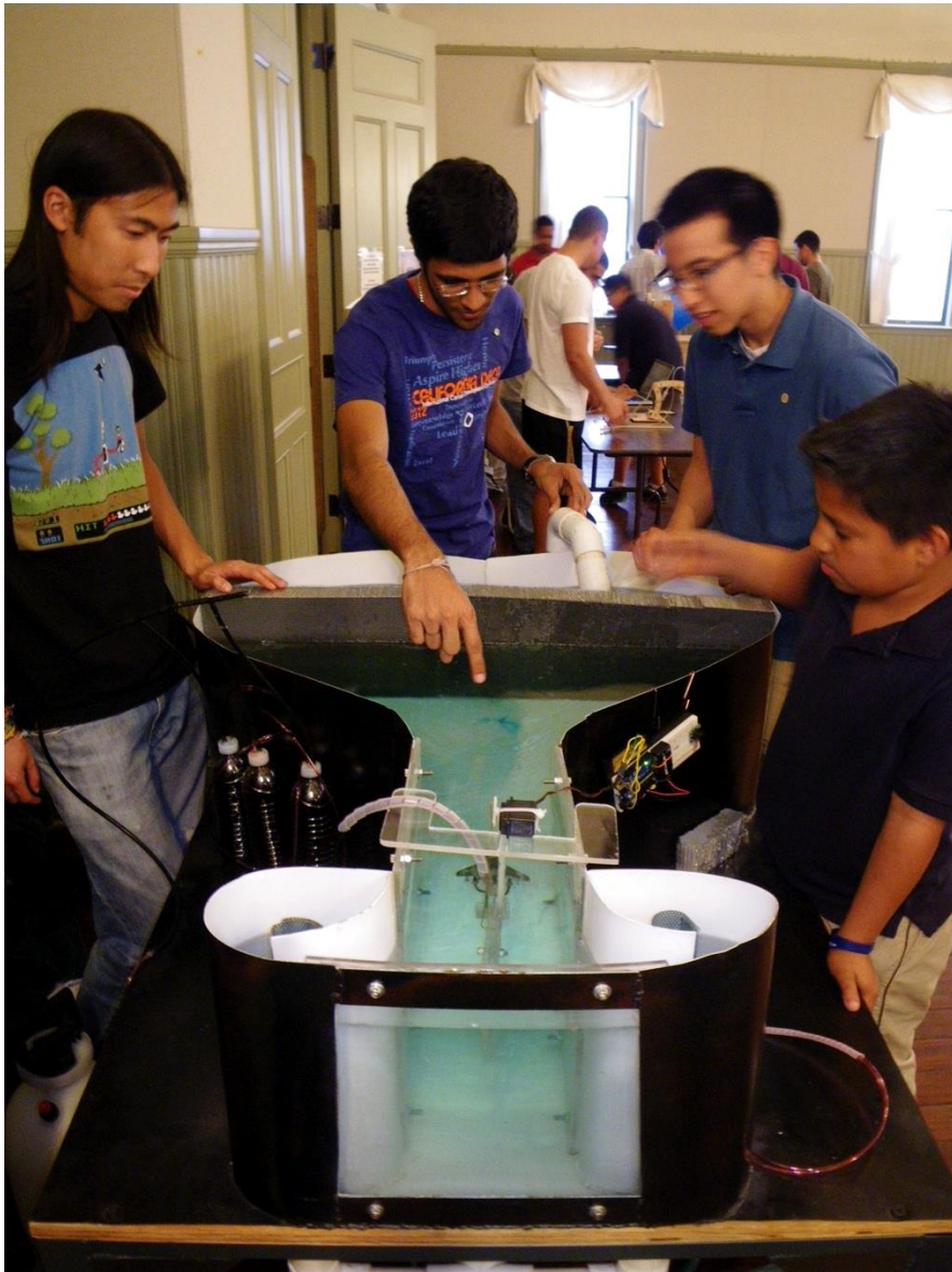
Figure 2: A 4 th -grader observing the flow streamlines around a model airplane in a portable water tunnel.
